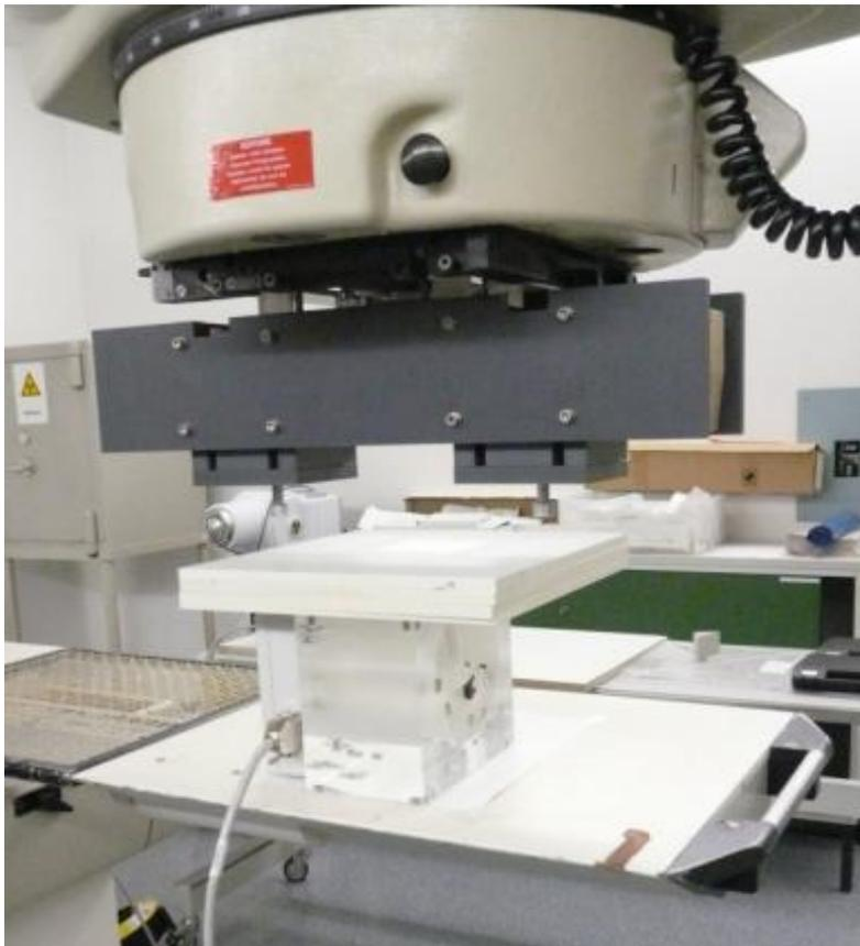
**Img 2: IC Dosimetric measurement setup with the preliminary model.**
