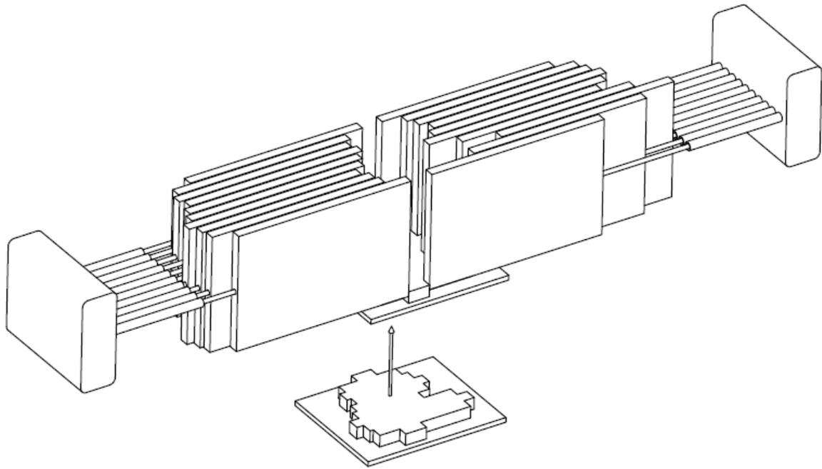
**Img 3: Concept of leaf drive with closed-loop pneumatic volume and stanchion and the insertion of an irregular field shape template for conformal treatment.**
