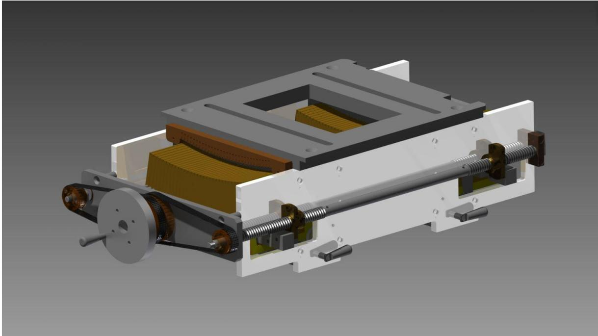
**Img 1: Drawing of the MLC without the pneumatic drive mechanism and the mounting plate**
